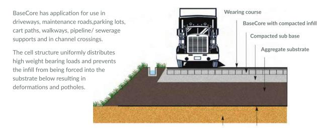
Existing substrate Non-woven Geotextile
