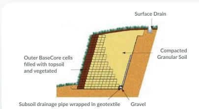
and barriers. The shear strength of the infill is enhanced by confining material within each cell. When installed in layers, BaseCore forms an integrated structural mass resisting lateral pressure and movement. BaseCore is easily dismantled and may be subsequently re-used.
